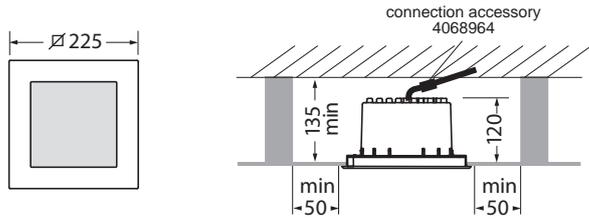
fixture for outdoor and indoor recessed ceiling installation.
