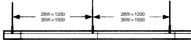
Mains Feed and Multiple Modules (Dimension from centre of mains feed)
